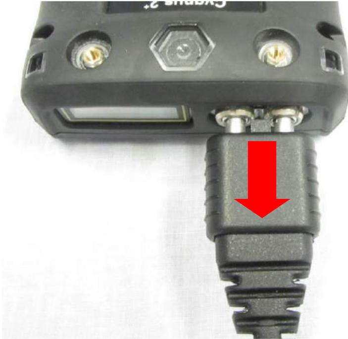
To release the connector simply pull back on the connector body. DO NOT pull the cable.
