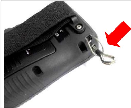
Wire loop fitted to the gauge body.
